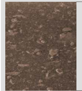
Injection moulded thermoplastic dry bearing material with additives homogeneously mixed in
